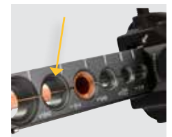
Laser etched sight gauge verifies proper flare
