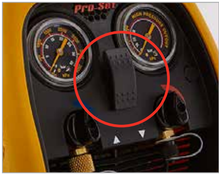
Ignition proof power switch
