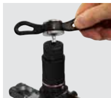
Ratchet handle with forward and reverse speeds flaring
