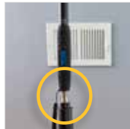
The EXP-64 can be mounted on tripods for longterm airflow analysis from wall or ceiling vents
