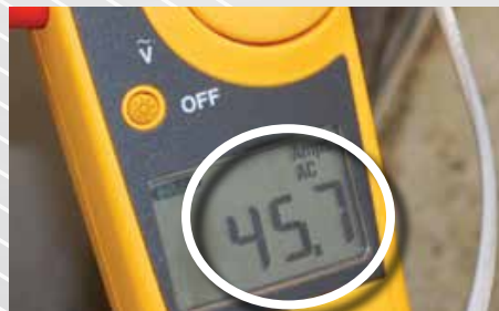
Amp measurement with 5-2-1 ® Compressor Saver ®
